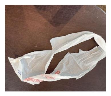
Probably the cutter stacked too many bags before cutting and they slithered. There's a slit in the side of the bag, "fringes" in the middle which interefere with weaving. The cut should be one smooth line. This cut piece is not useful and will be recycled.
